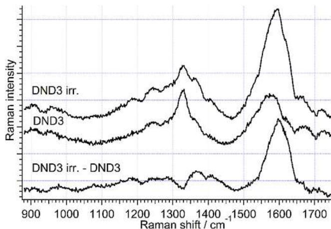
Fig. 7. The effect of nitrogen ions irradiation on the ND structure: Raman spectra under 355 nm excitation of irradiated sample (top), original sample (middle), and the difference (bottom).
