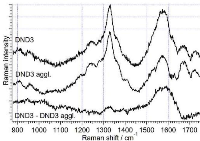
Fig. 5. Raman spectra under 355 nm excitation of de-agglutinated DND3 (top), initial agglutinates (middle) and the difference (bottom).
