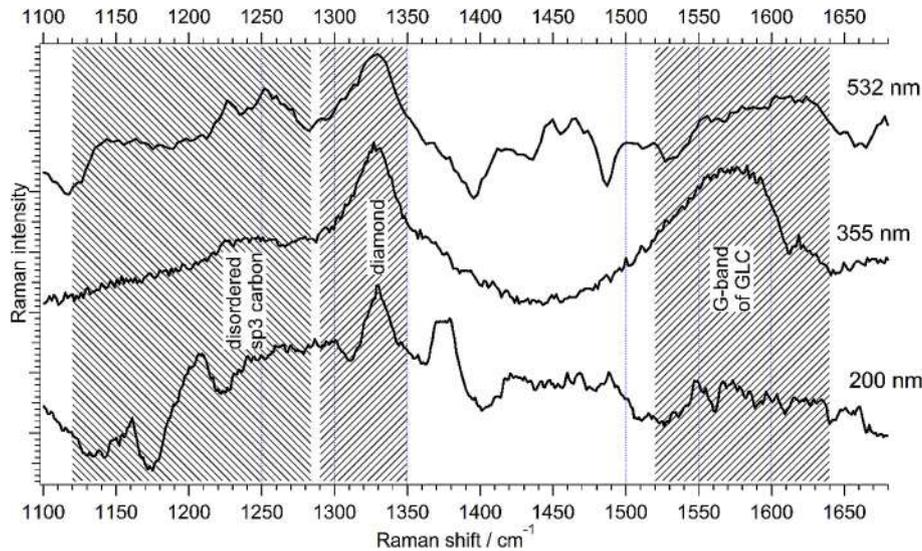
Fig. 1. Experimental Raman spectra of 3 nm DND at different excitation wavelengths; the major bands of different carbon phases highlighted.
