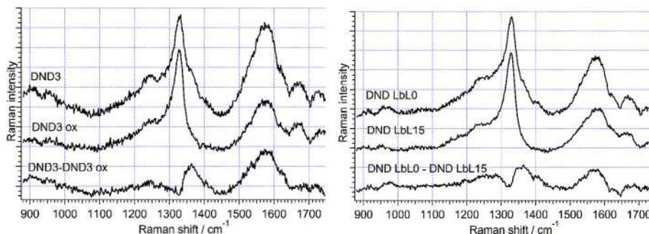
Fig. 6. Oxidation of ND by air (left) and layer-by-layer etching (right). Top curves: spectra of original samples, middle: oxidized, bottom: difference. The Raman spectra were measured under 355 nm excitation. (A colour version of this figure can be viewed online.)
