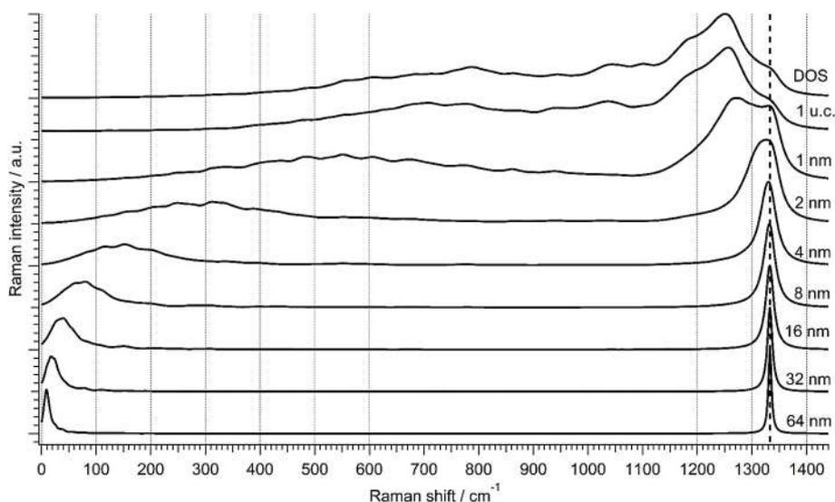
**Fig. 2.** Calculated Raman spectra for different confinement lengths starting with disordered sp<sup>3</sup> carbon network (DOS), next is 1 unit cell (1 u.c.) confinement (i.e. 0.3567 nm). The dashed line indicates the frequency at the  $\Gamma$  point (1332.9 cm<sup>-1</sup>).
