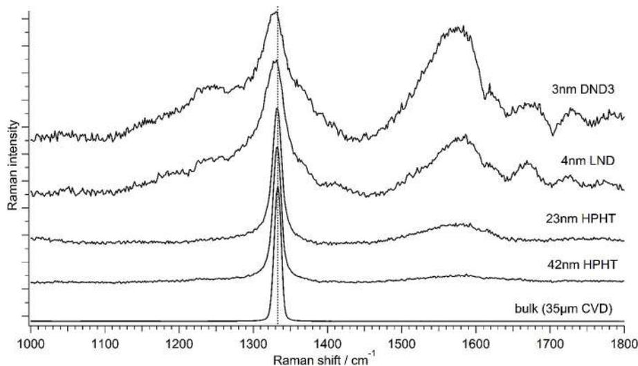
**Fig. 3.** Representative Raman spectra of ND samples of different mean size and origin under 355 nm excitation. Size in this figure is given as estimated by DLS for HPHT and DND3 samples and by XRD for the LND one. The position of the zone-center phonon ( $1332.9 \text{ cm}^{-1}$ ) is indicated by the dotted line.
