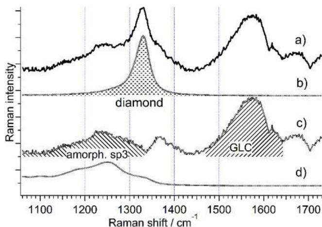
**Fig. 4.** The procedure of analyzing the ND spectra: the experimental spectrum (a), fit of the diamond band with PCM equation (b), ND spectrum after subtraction of the diamond band (c), DOS of diamond shown to confirm assignment of the amorphous diamond band (d). (A colour version of this figure can be viewed online.)
