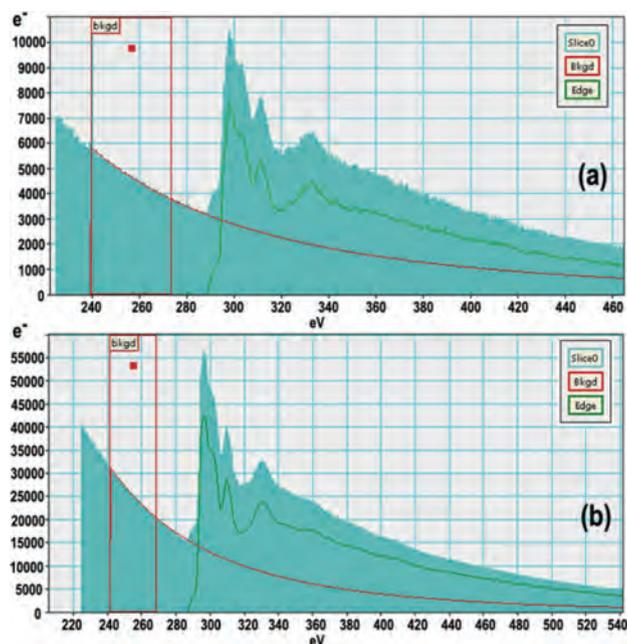
**Figure 4.** Electron Energy Loss Spectroscopy (EELS) (a) DND, (b) LND.
