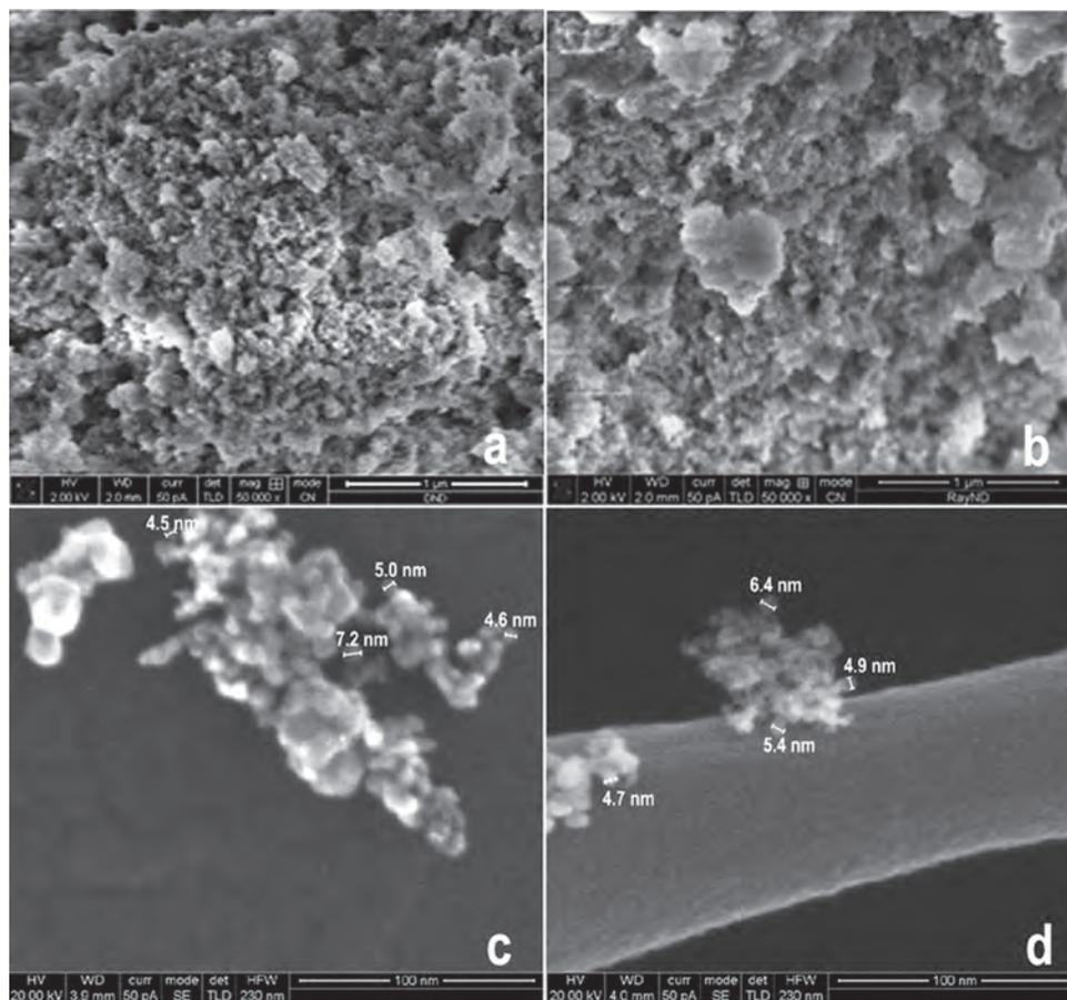
**Figure 2.** High Resolution SEM images of DND (a) and (c) and LND (b) and (d); the scale bar in (a) and (b) is 1  $\mu\text{m}$ , in (c) and (d) 100 nm.
