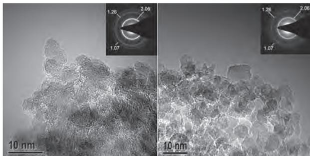
**Figure 3.** HR TEM images and selected area electron diffraction patterns (SAEDs) (insets) acquired from DND (left) and LND (right) nanodiamond specimens.
