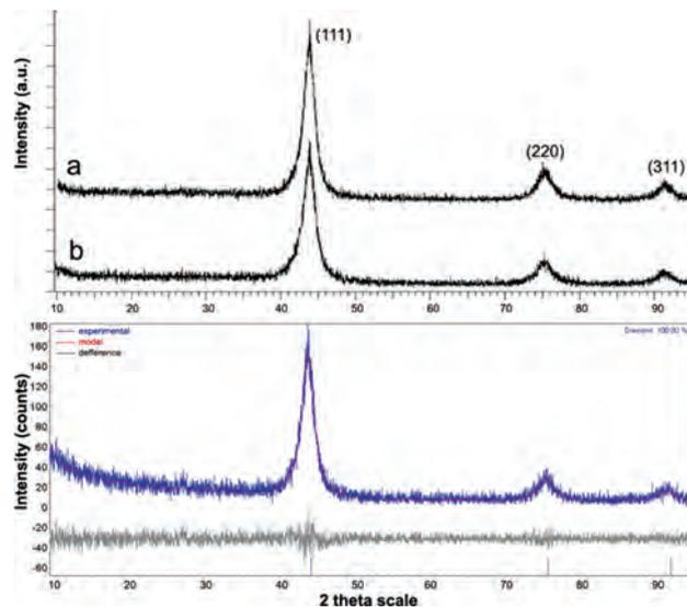
**Figure 1.** XRD patterns acquired from nanodiamond powders (a)—specimen LND, (b)—specimen DND) (upper) and graphical representation of Rietveld refinement results for nanodiamond synthesized by LHDP method. Peak positions of Diamond are shown by vertical bars (bottom).
