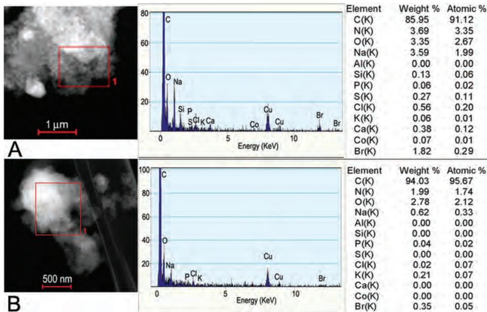
**Figure 5.** Energy Dispersive X-Ray Spectroscopy (EDS) (a) DND, (b) LND, the analyzed area (left), energy Dispersive X-Ray Spectra (middle) and elements quantity (right).
