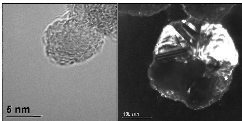
**Figure 5.7** HRTEM images of LND on the left and LND obtained under an enhanced pulse width on the right.
